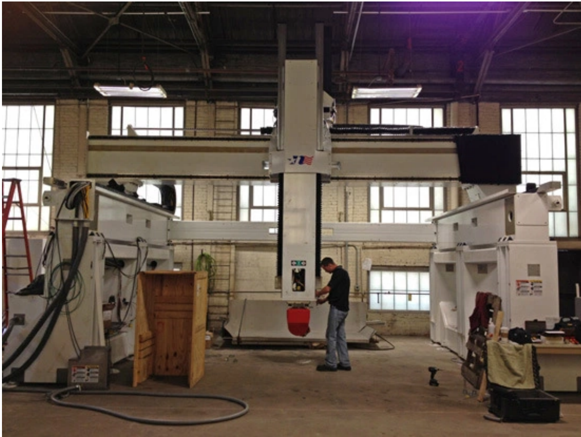
Computer Controlled Stone Milling Machine – Installation
